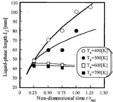
**Fig. 11** Liquid-phase length ( $L_i$ ) variation for ambient temperature change
