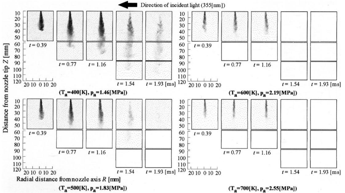
**Fig. 10** Liquid-phase images with exciplex fluorescence method using 35 mm still camera ( $p_{inj}=72$  [MPa]  $Q_{inj}=12.0$  [mg]  $\rho_a=12.3$  [Kg/m<sup>3</sup>])
