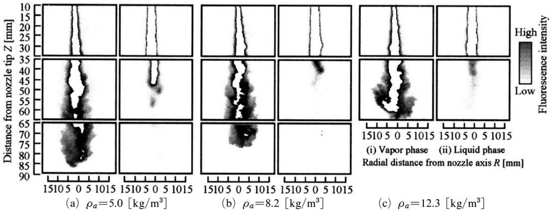
Fig. 7 Temporal change in free diesel spray with exci-plex fluorescence method
