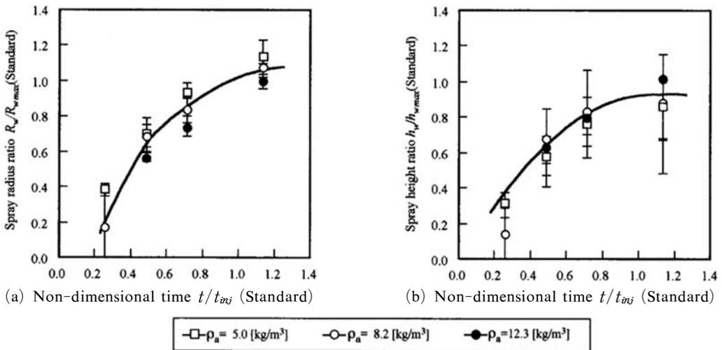
Fig. 5 Temporal change in spray radius  $R_w$  and height  $h_w$
