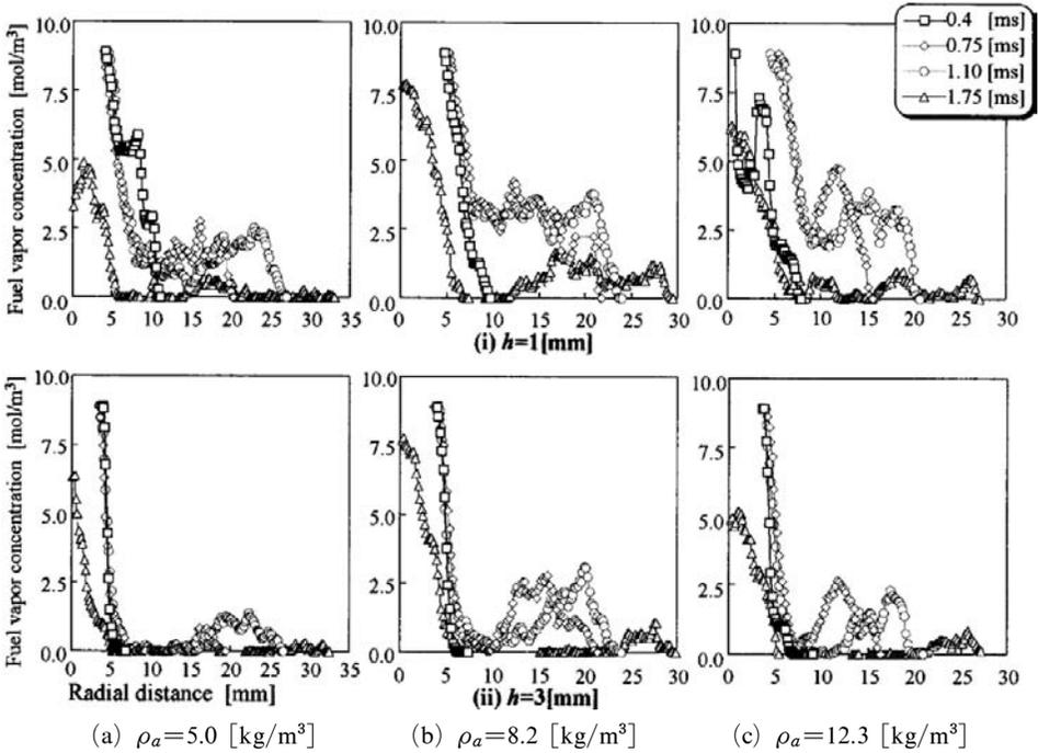
Fig. 6 Radial distribution of fuel vapor concentration
